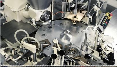
As an option we supply a machine with new Easy opening system (tear cell) for inserting of red tape into a packed portion for easy opening of the portion.
