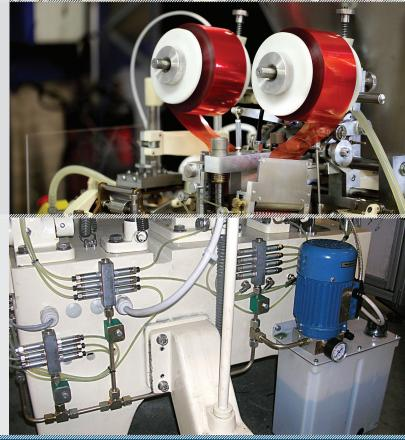
As an option we supply automatic central lubrication system integrated in the packaging machine.
